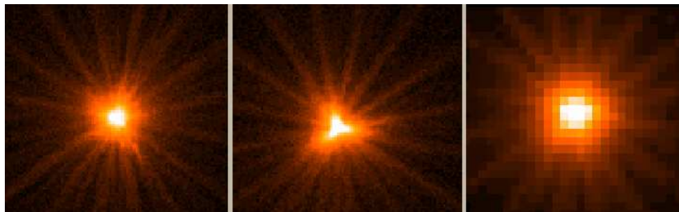
Figure 3.4: On axis point spread function of the MOS1, MOS2 and pn X-ray telescopes (left to right) registered on the same source, with each MOS camera in Small Window Mode, and the pn camera in Large Window Mode (see Section 3.1). The star-like pattern is created by the spider which supports the 58 co-axial Wolter I mirrors of the telescope. The shape of the point spread function core is slightly different for all cameras, with MOS2 having a somewhat triangular shape. Figure adapted from the XMM – Newton Users’ Handbook .
