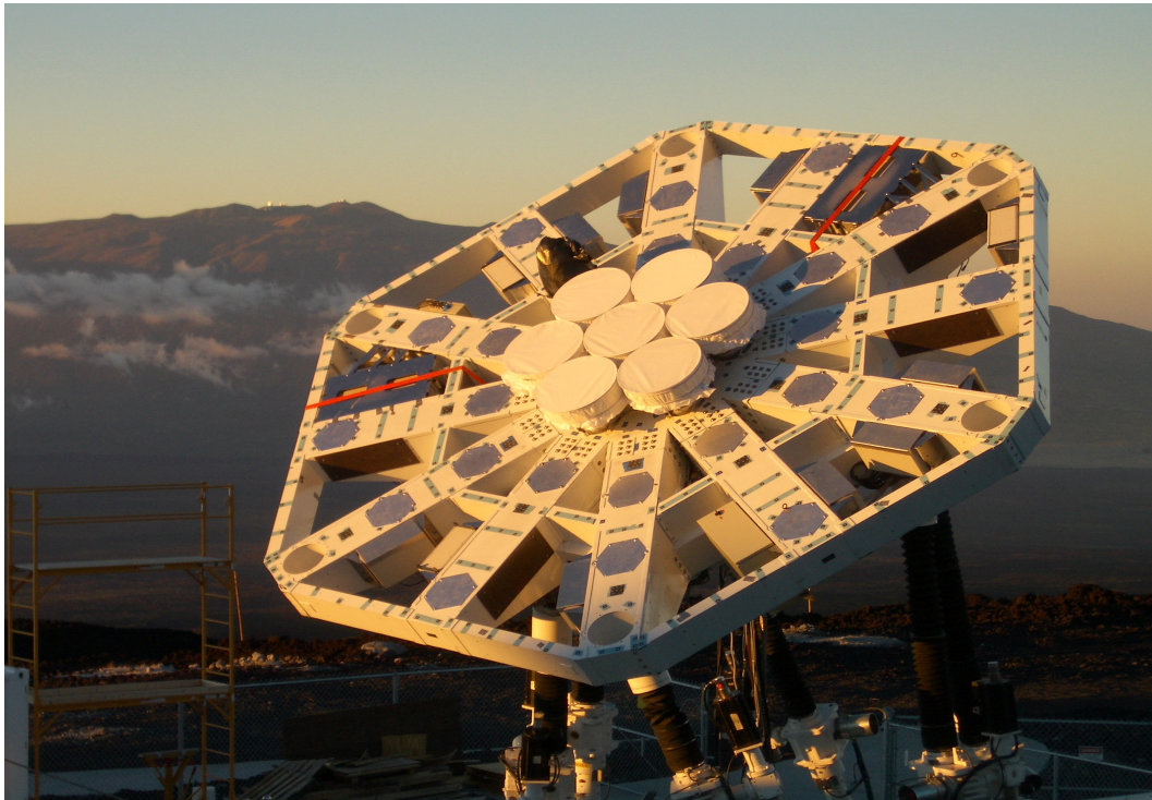
Figure 2. AMiBA with its initial 7-element configuration with 60cm reflectors operating on Mauna Loa.
